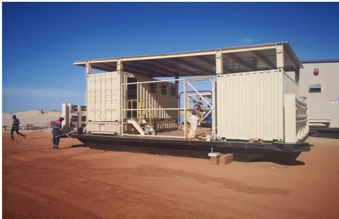
THE MOBILE MAINTENANCE SKID — DRAGGED ACROSS THE SAND BY BULLDOZER
