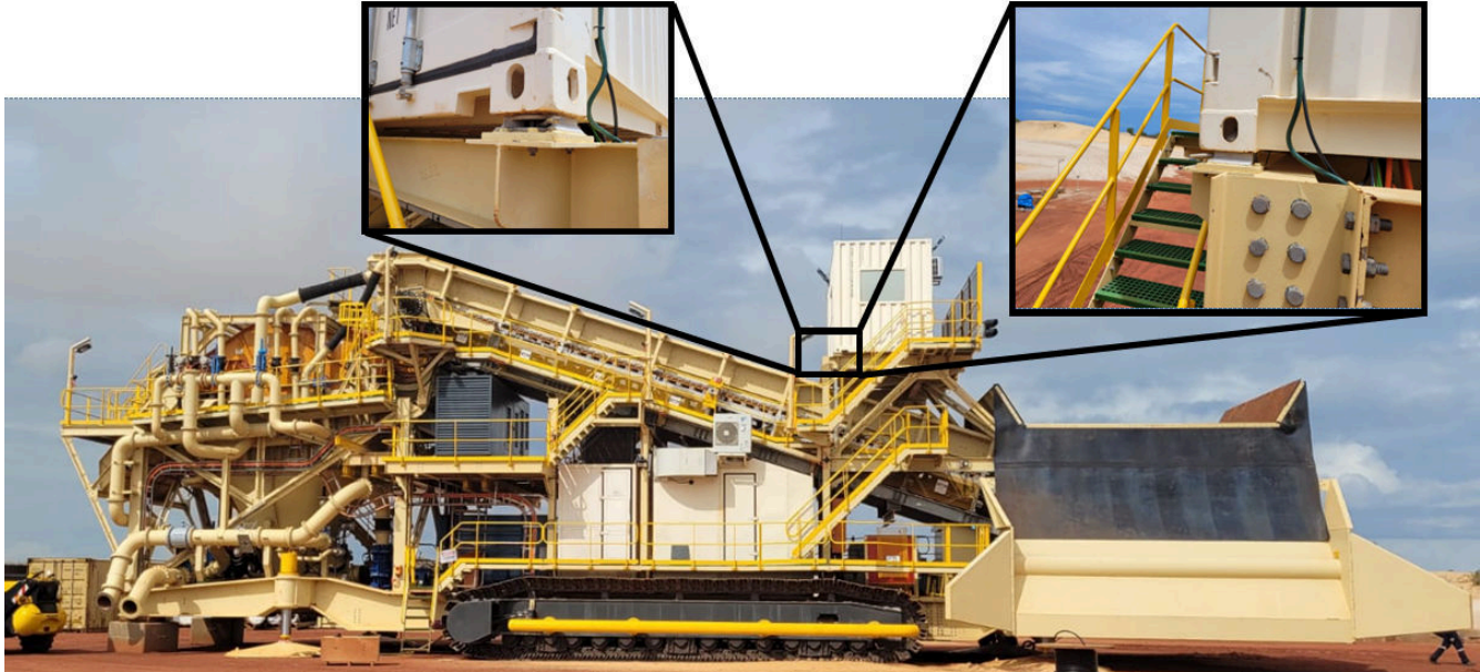
THE DRY MINING UNIT ON SITE — INSETS SHOW THE CONTAINERISED CONTROL ROOM AND ITS BOLTABLE TWISTLOCK FIXINGS
