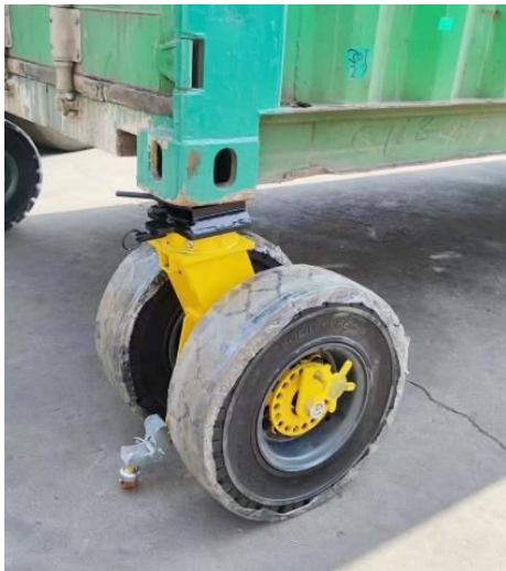
DOVETAIL TWISTLOCK ENGAGED IN THE CORNER CASTING
