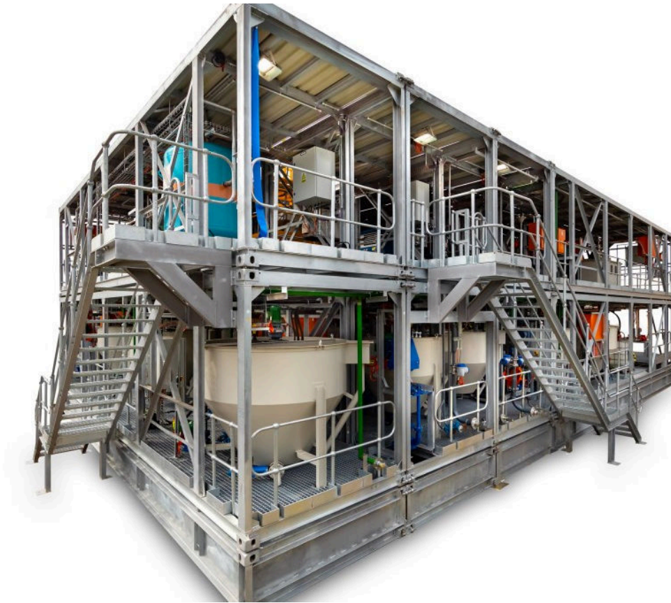
MODULAR FINES-FLOTATION PLANT — TRANSPORTABLE ISO-FRAMED SKIDS
